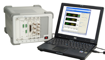
U2722/3A used as a modular instrument
